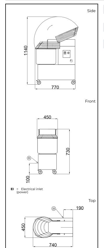
Electric 380-415V/3 ph/50 Hz Supply voltage: **Total Watts:** 1.1 kW Capacity: Maximum kneading (60% 25 kg/Cycle hydratation): Key Information: External dimensions, Width: 450 mm External dimensions, 740 mm Depth: External dimensions, Height: 730 mm 86 kg **Shipping weight:** 33 lt **Bowl capacity:**
